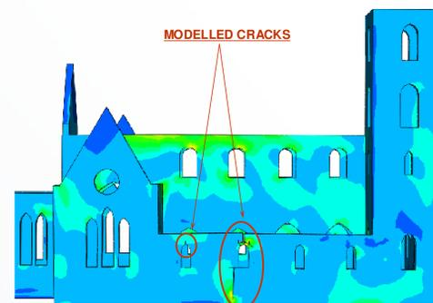
Fig 6 : Cracked model of the church, max principal stress
