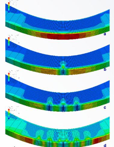
Fig 5 : Major steps in the crack propagation process in a test beam (a, b, c), final step (d), max principal stress
